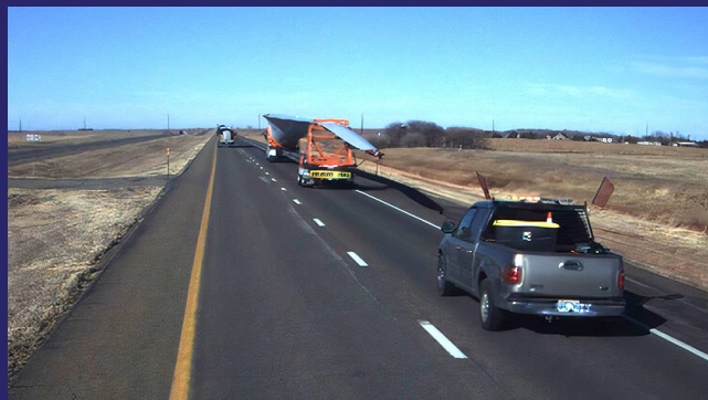
Example: Turbine blade followed by chase vehicle with flashing lights.
