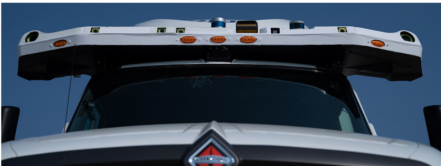
Roof sensor beam on experimental driverless prototype.
